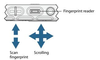
You can use the OmniPass application to associate your fingerprint with passwords for Web pages and other applications. You can also use the fingerprint reader as a scrolling device. Move your finger on the fingerprint reader to move the pointer on the screen.
